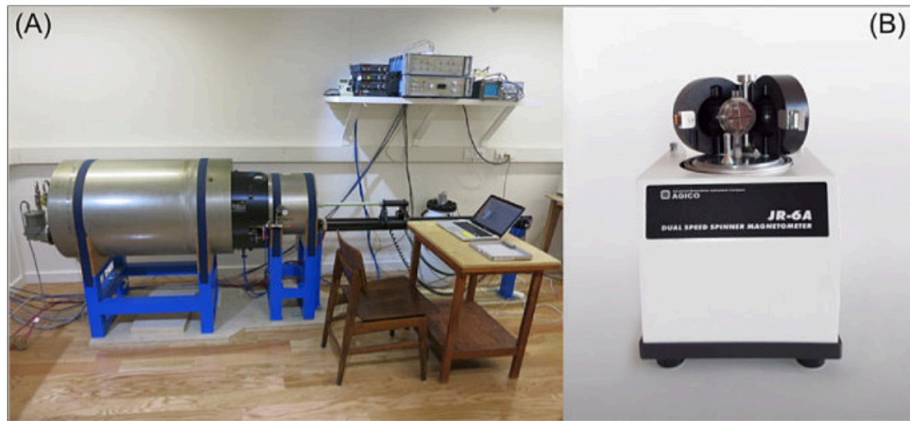
Figure 7. (A) Cryogenic magnetometer 2-G (Source: https://scholars.huji.ac.il/ronshaar/2g-srm-magnetometer ). (B) Spinner magnetometer JR6 AGICO (Source: https://www.agico.com/text/products/jr6/jr6.php ).
